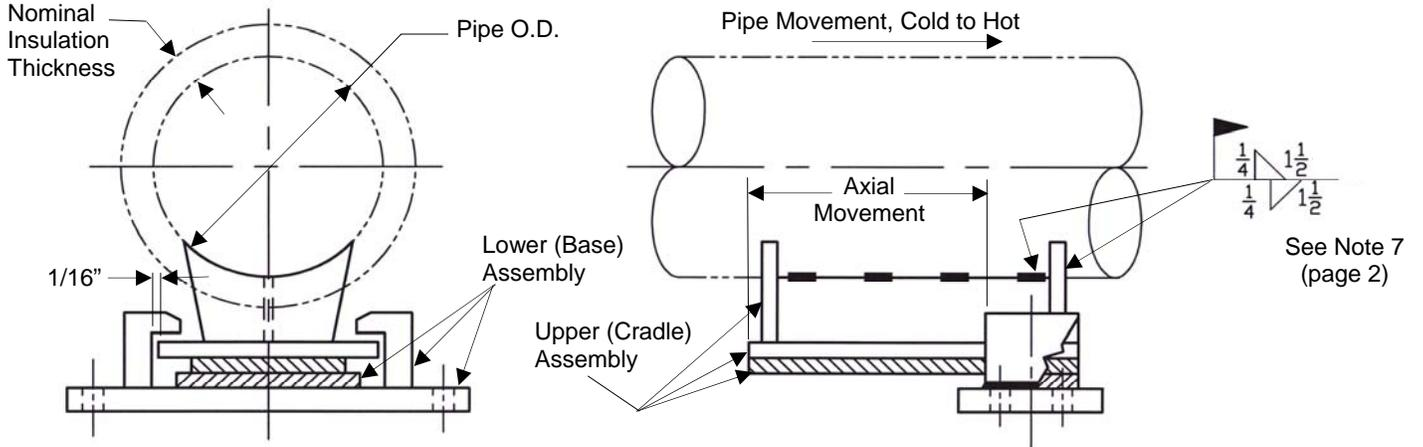
**Figure 2 - "101-B" Low Friction Graphite Guide**
