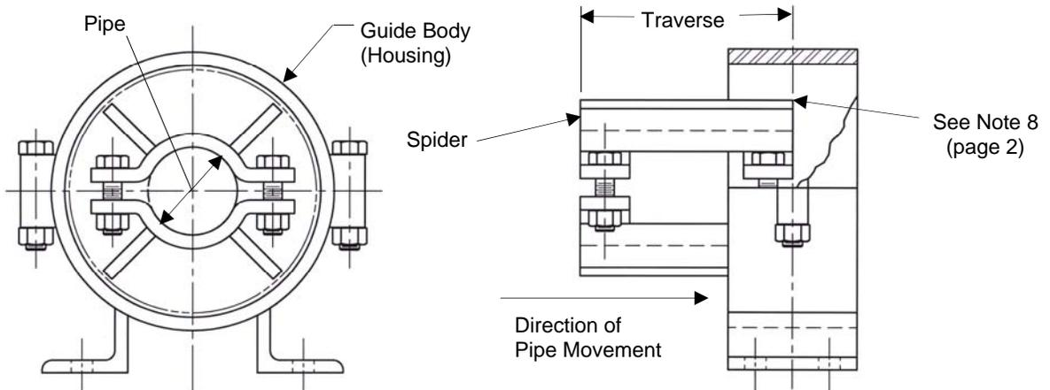
**Figure 3 - Radial Alignment Guide**
