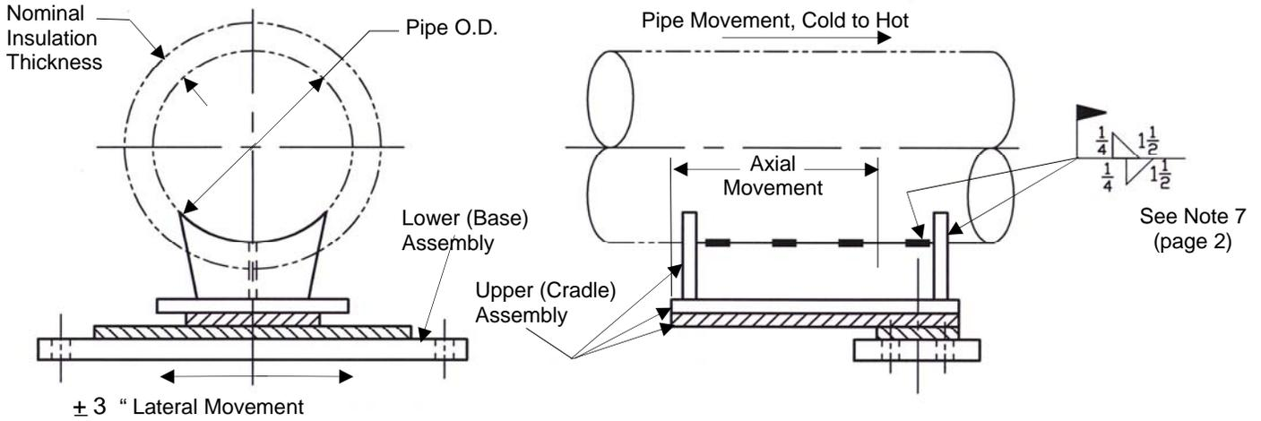
**Figure 1 - "201-B" Low Friction Graphite Support**
